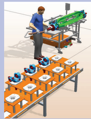
Dynamic Assembly Lines with Conveyors, Carriers, AGVs
